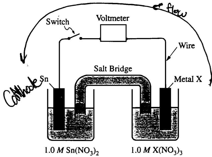
6. An electrochemical cell is constructed with an open switch, as shown in the diagram above. A strip of Sn and a strip of an unknown metal, X, are used as electrodes. When the switch is closed, the mass of the Sn electrode increases. The half-reactions are shown below.
