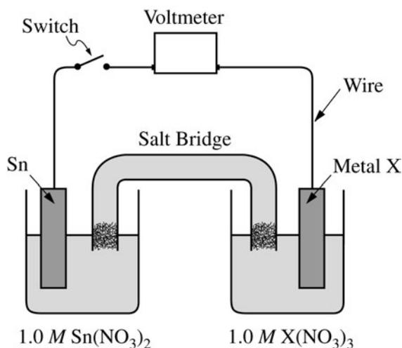
An electrochemical cell is constructed with an open switch, as shown in the diagram above. A strip of Sn and a strip of an unknown metal, X, are used as electrodes. When the switch is closed, the mass of the Sn electrode increases. The half-reactions are shown below.
