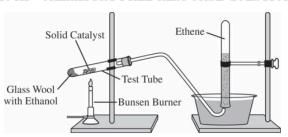
2. Ethene,  $C_2H_4(g)$  (molar mass 28.1 g/mol), may be prepared by the dehydration of ethanol,  $C_2H_5OH(g)$  (molar mass 46.1 g/mol), using a solid catalyst. A setup for the lab synthesis is shown in the diagram above. The equation for the dehydration reaction is given below.
