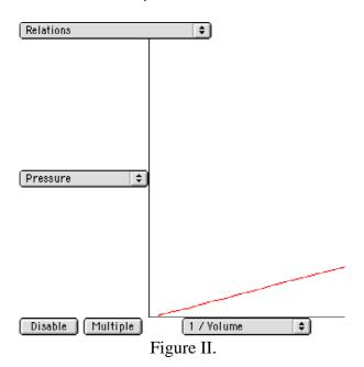
Clicking on the Enable button causes a change in the Control Bar Region, activating the pressure and volume scrollbars, and deactivating the mol and temperature scrollbars. Moving either the pressure or volume scrollbar will generate a plot of those two variables in the Plotting Region. What kind of plot is shown? The Multiple button allows two or more plots to be superimposed.
